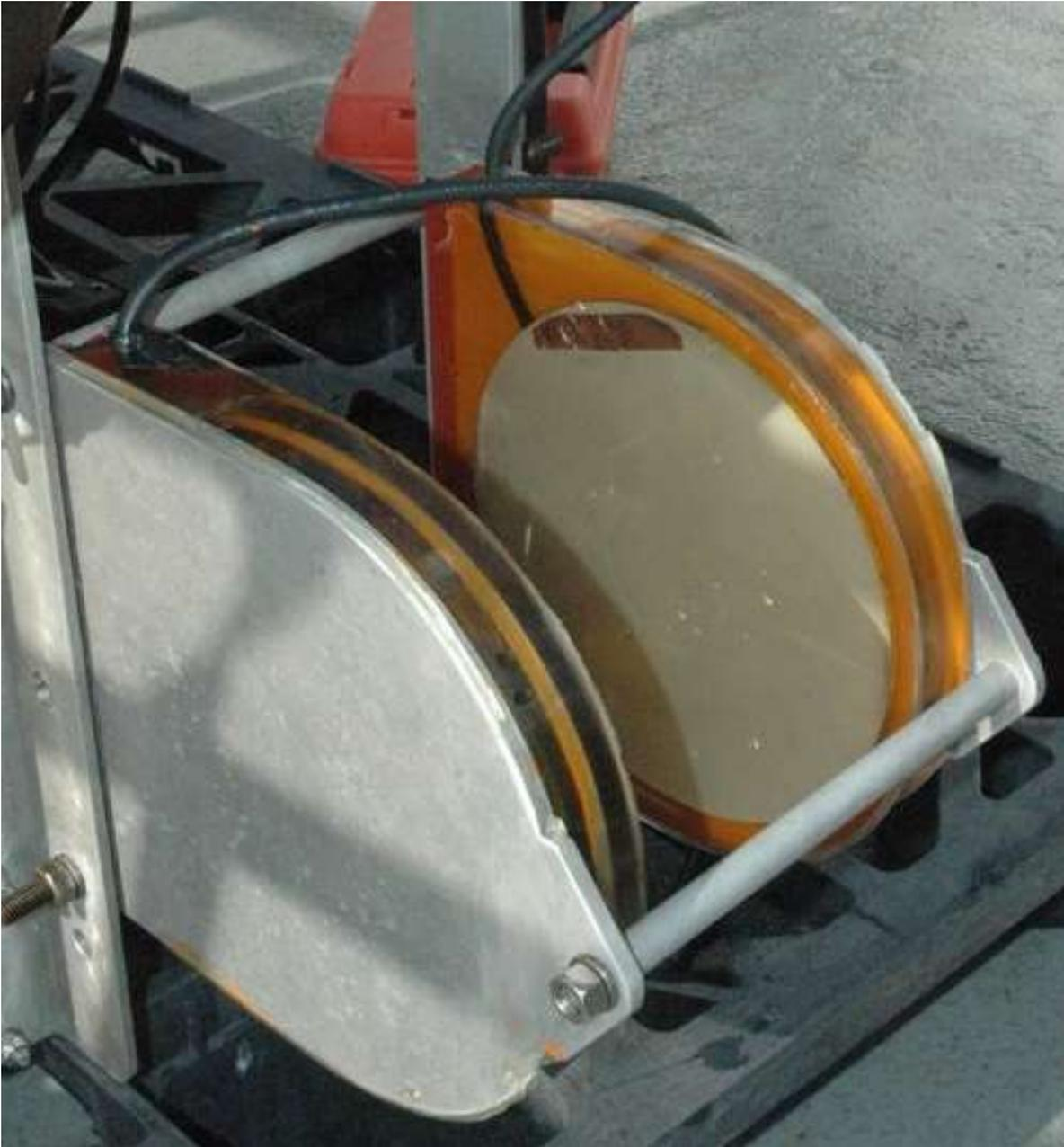
*Figure 1: Redesigned resonator designed to operate at frequencies up to 1 MHz attached to the MASCOT package for deployment from R/V Kilo Moana on the Hawaii cruise.*
